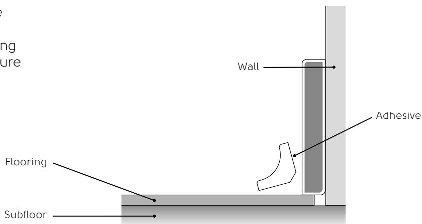
Use finishing nails every 450mm (16") through the scotia into the skirting. Be sure to pre-drill any holes.
